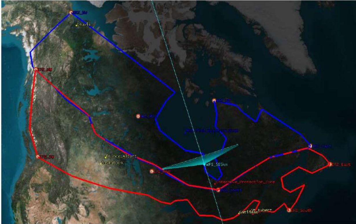
Figure 3-1: WFS operation concept diagram. The ground track of a satellite is shown, along with the expected swath coverage width (teal colour). The red area is the IPZ, and the blue area is the MRZ. Yellow labels show the 5 Govt ground station locations.
